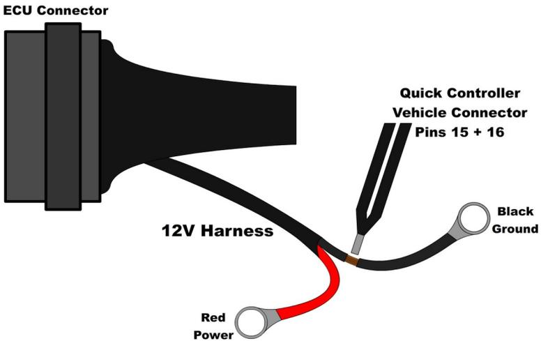
**Step 2: Install the adapter between the throttle position sensor and the ECU wiring harness.**
